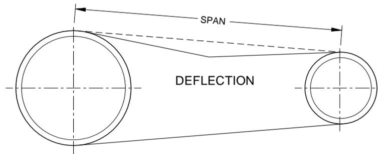
**⚠ CAUTION:** Excessive belt tension is the most frequent cause of belt wear, bearing wear and noise.
