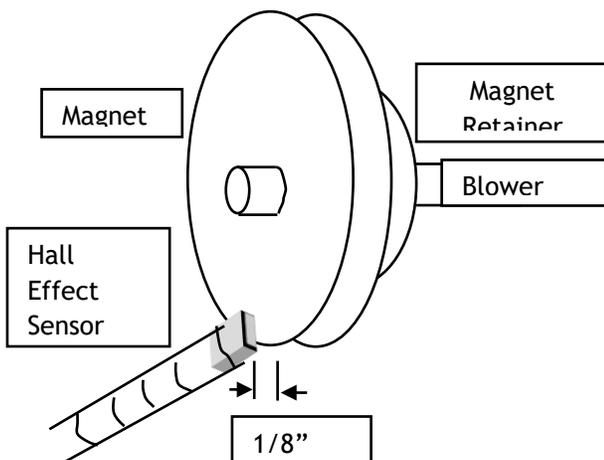
With a digital AC voltmeter, measure the AC volts present on terminals "YS to GS". When the combustion blower is running there should be 4 to 6 Vac present. If the AC voltage is not present, check the tachometer sensor to magnet gap. It should be 1/16 to 1/8 inch. If the gap is satisfactory, attempt to repair by flipping the
