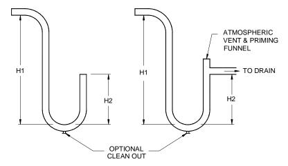
Ensure adequate clearance for properly sized drain traps.
